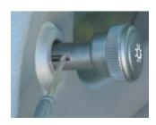
Pull the existing factory headlight knob out to the "ON" position. Insert a small flat headed screwdriver into the slot on the side of the headlight knob. Gently pry on the retainer clip while pulling on the knob. The knob will simply slip off the mounting post once the clip is disengaged.
