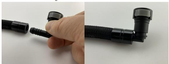
When installing check valves, be sure to note the direction of flow. UPR check valves have arrows printed on them. **The arrow always faces AWAY from the catch can** when installed in the vacuum hose.
