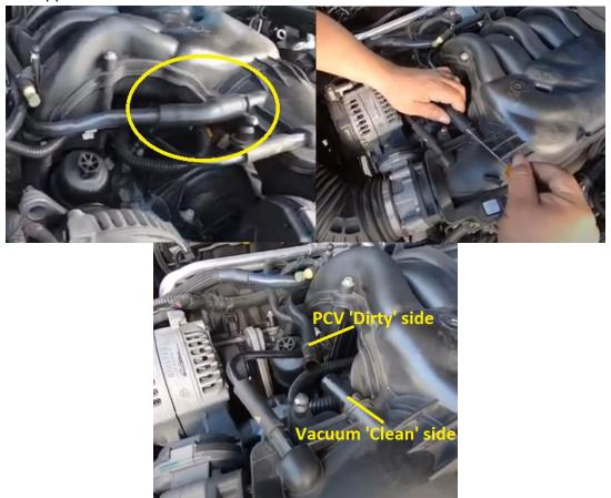
2. Remove the intake cover and locate the PCV tube. Remove the rubber boot (circled) connecting the tube to the intake manifold vacuum port.
