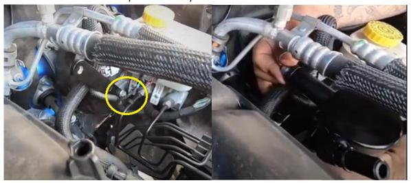
1. Remove the inside nut securing the master cylinder to the brake booster. Attach the UPR catch can bracket to the stud and secure it with the factory nut as shown (circled). Install the UPR catch can using the supplied Allen bolt and washer.
