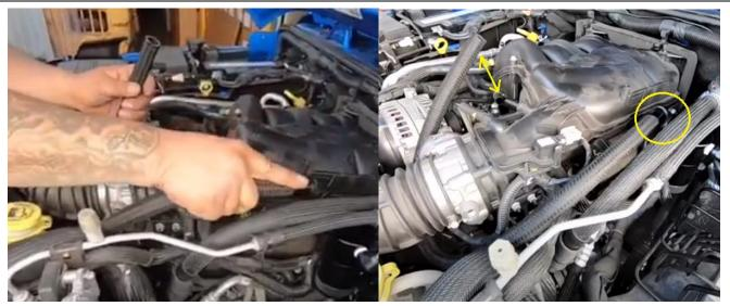
3. Using the shorter of the two hoses, rout the hose under the intake tube. Slide the UPR billet hose end onto the bare end of the hose and push it onto the plastic PCV tube. Connect to the inside fitting on the catch can using the UPR Plug n Play fitting. The fitting will click on when properly engaged.
