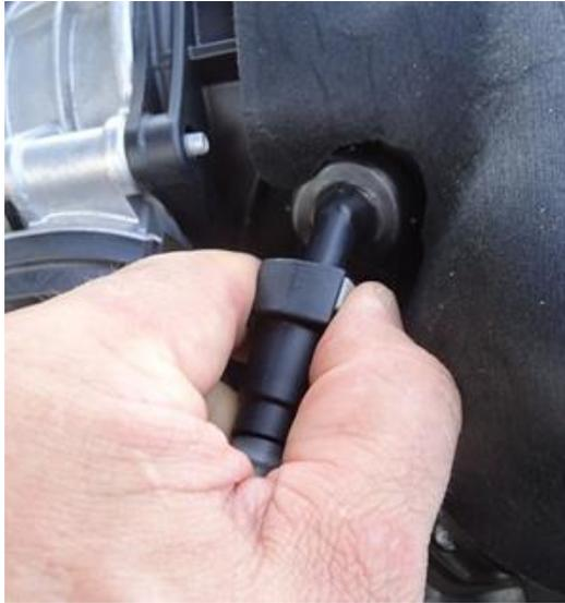
2. Remove the bolt from the large ground wire right above the steering knuckle on the driver side inner fender well. This is the one that is just to the LEFT of the ground wire that is directly across from the spark plug wire. Make sure the L bracket on your catch can is facing down. Install the supplied longer stud, lock washer, catch can and tighten in place. See stud instructions in the next step.
