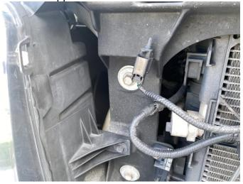
2. Install the provided bolt into the hole where the ACT sensor was removed. Install the catch can bracket onto the bolt and use an allen wrench to securely fasten the catch can.
