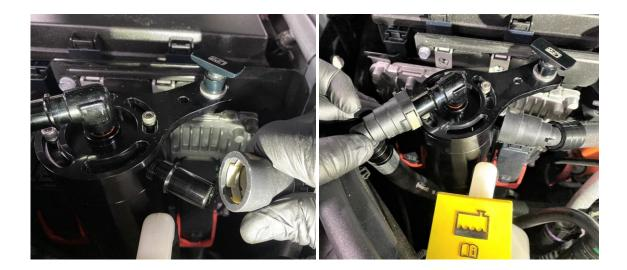
5. Install the UPR catch can onto the 90-degree billet bracket with the supplied bolt. Install the UPR Plug N Play™ Fittings onto the catch can. The 'Dirty' side hose will connect to the Top of the catch can. The 'clean' side hose will connect to the right side of the catch can.
