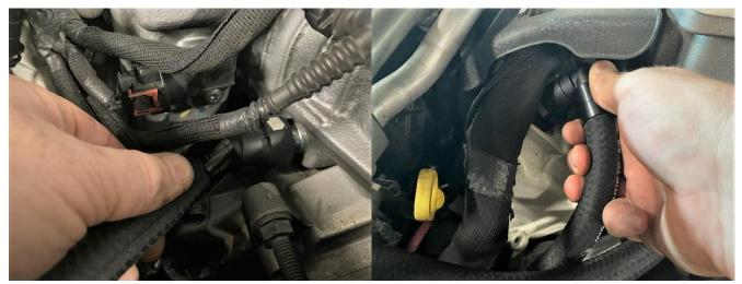
4. Install the hoses onto the engine by pushing the UPR Plug N Play™ female fittings onto the vacuum and PCV male fittings until they click.
