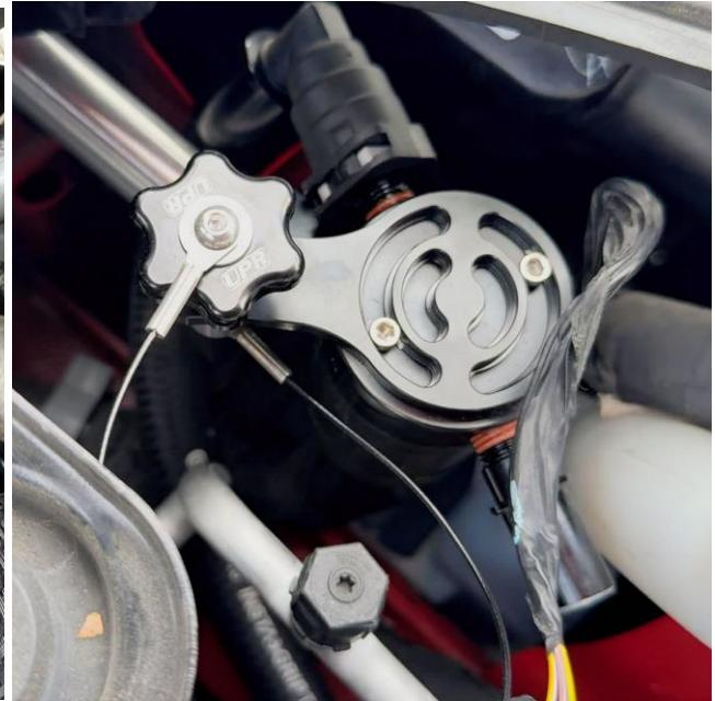
4. Attach the UPR hose with the male fitting to the hose from the valve cover. Attach the 90 degree end of the hose to the rear facing fitting on the catch can (Routing the hose under the catch can).
