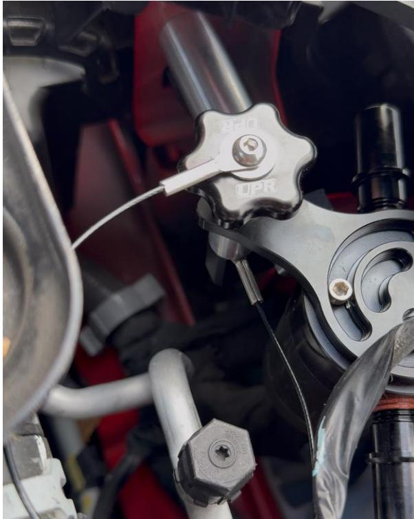
3. Install the Clean Side Catch Can onto the UPR billet bracket. Leave the quick release knob and bracket screws a little loose so you are able to position the catch can for the best fit.
