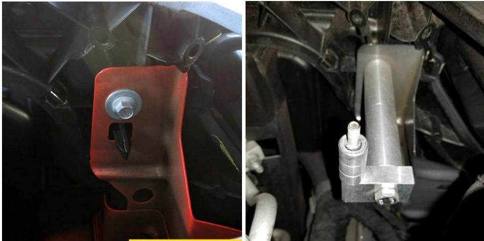
1. Locate the bolt at the radiator support behind the passenger headlight. Remove the bolt and install the UPR Billet bracket as shown.
