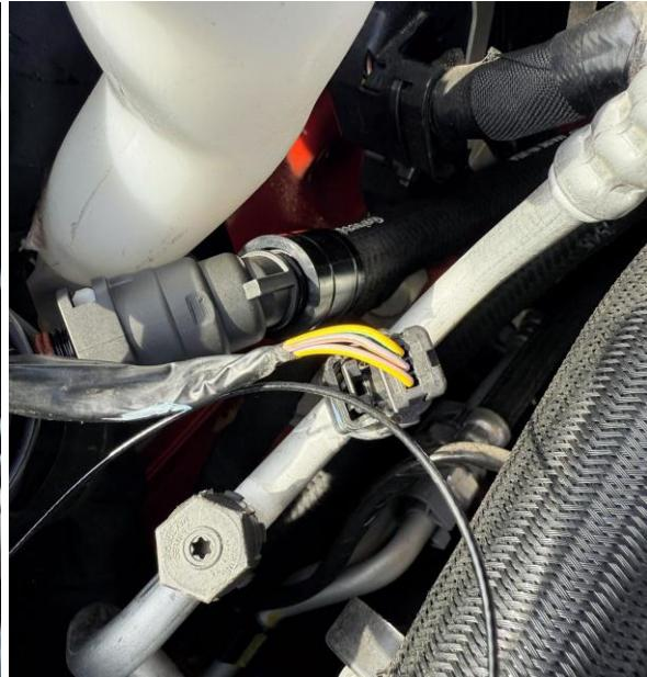
5. Connect the remaining hose to the air intake tube (90 degree fitting) and route the hose towards the catch can. Connect the 45 degree fitting to the front facing fitting on the catch can. Be sure to route the hose avoiding any hot exhaust and secured from any hazards.
