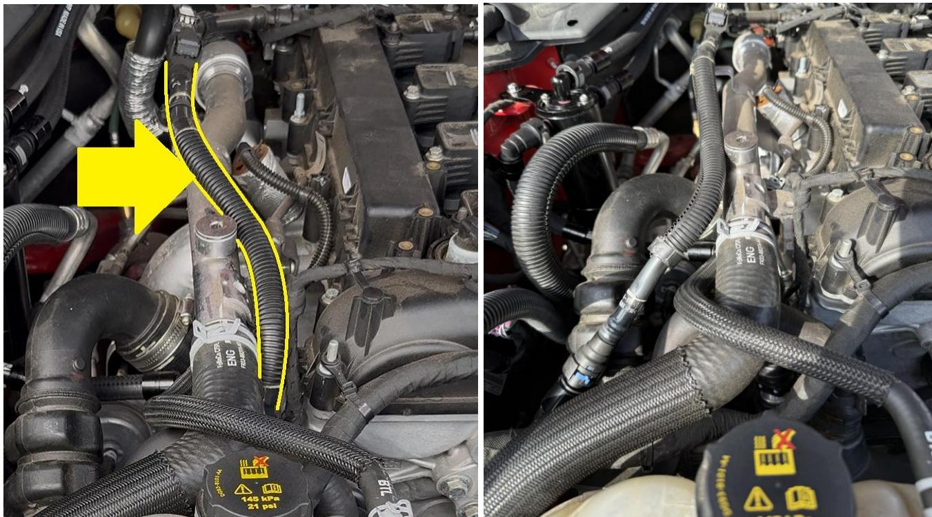
2. Locate the Crankcase Vent (CCV) Tube at the left rear of the valve cover. Follow the hose from the valve cover to the turbo inlet tube. Disconnect the hose from the turbo inlet tube and twist it so that it points towards the passenger side as shown. The hose will swivel at the sensor connection.
