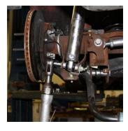
Remove the bolt holding the bottom of the shock in place and move it to the side, repeat on opposite side.
