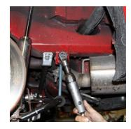
Remove the bolts holding the factory sway bar link to the body, repeat on other side.
