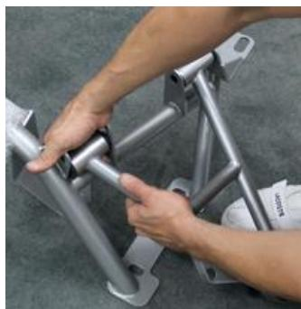
Lastly pull the front of the A-arm into place and align with mounting bolt holes.
