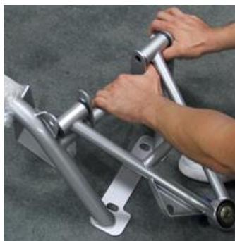
Now you can pull rear side of the A-arm in place to align with mounting bolt holes.
