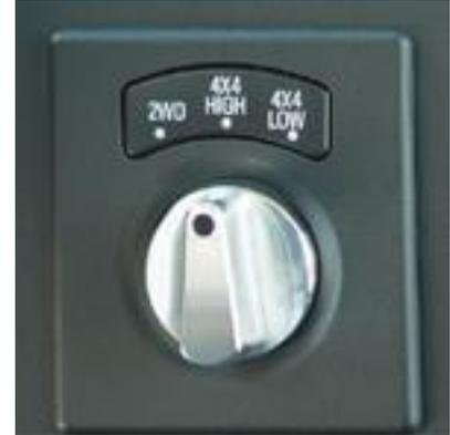
1. Remove the factory 4x4 selector knob by pulling straight back on it.
