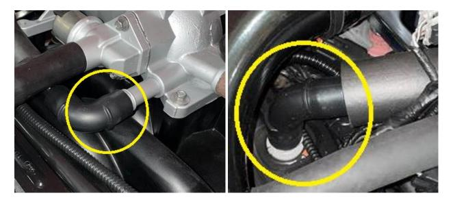
**2.** Locate and remove the factory PCV hose. It will run from the vacuum fitting on the front side of the throttle body to the PCV fitting on the passenger side valve cover.
