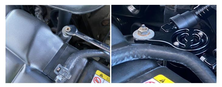
**1.** Remove the factory nut on the coolant bottle tank. Install the UPR catch can bracket onto the stud and reinstall the nut.
