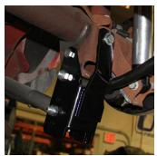
12. Install the Passenger side bracket. The 12mm bolt goes into the top bolt hole or reinstall the factory axle weight. Put the 14mm x110 bolt with spacer through the second hole. The back strap is secured with ½ bolt, washer and nut. The control arm bolts in with 14mmx110 bolt.
