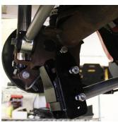
9. The two relocation brackets will have a short and tall side the short side faces outwards towards the tires. Slide the Driver side into place and insert the 14mm x 110mm bolt with spacer through the second from the top bolt hole.
