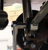
8. Unbolt the pan hard bar bolt but do not remove it just back it out till the factory nut comes off but you can leave the bolt in to keep the bar in place.
