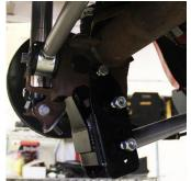
11. Next push the factory pan hard bolt through the relocation bracket back strap and tighten using the factory nut.
