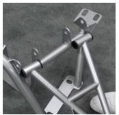
\*Now you can slowly rotate the other end of the A- arm towards the back slot of the K-member. Stay well below the mounting bolt holes.
