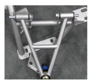
Proper bolt alignment using UPR's Grade 10.9 Hardware Kit.
